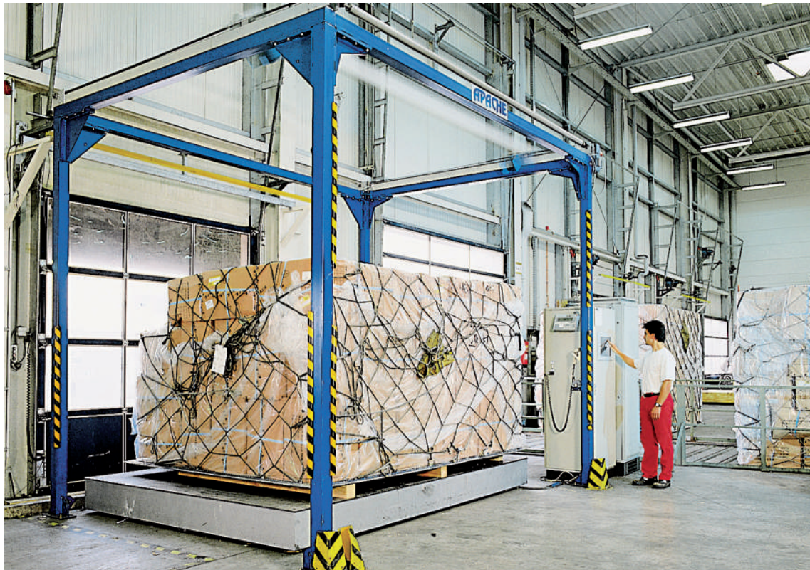
Volumenportal, Bodenwaage Staplerbeladung
